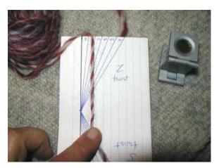
This picture illustrates measuring the twist angle of a singles yarn. I've anchored the yarn in a small slit at the top of the card, and I hold it straight, parallel to the lines on the card, with my finger. Don't pull it tight—just hold it under enough tension to keep the yarn reasonably straight. More tension than that will stretch the yarn, making the angles measure more shallow than they really are.
